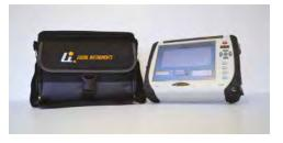
The LOR family now has options for built-in optical power meter (OPM), visible (red) fault locator (VFL) and a USB connector inspection microscope add-on with a wide range of different connector adapter tips, so connector end face images can be viewed on the OTDR screen and saved in internal memory or external drives.
