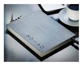
With comprehensive IP packet analysis tools, NOMAD is ideal for IP transport understanding regardless of media transported. NOMAD also is shipped with the ultimate in user friendly setup. The unit contains a Wi-Fi zone, and by pointing a laptop towards this, NOMAD is ready for use without further configuration.
