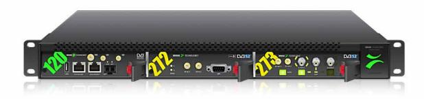
The VB273 has multiple layers of redundancy. The 1RU chassis offers dual redundant power supplies and the VB273 switching card has magnetically latching relays to protect against signal disruption, even during a complete loss of power.
