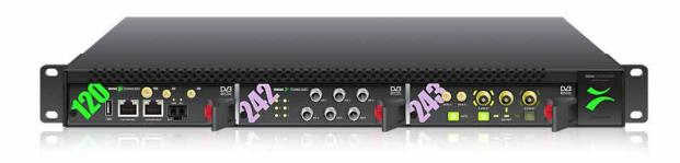
The VB243 INTELLIGENT REDUNDANCY SWITCH has multiple layers of redundancy. The 1RU chassis offers dual redundant power supplies and the VB243 switching card has magnetically latching relays to protect against signal disruption even during a complete loss of power.
